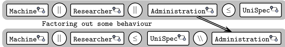
Fig. 6. One possible step in Stepwise modularisation of requirements: Factoring out the behaviour of the Administration.
