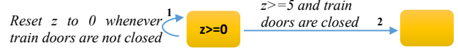
Fig. 4 Conductive graph. Each rectangle denotes one state. The edge between states is considered as a state transition. The constant numbers (e.g., 1 and 2) near transitions denote the priorities for transitions
