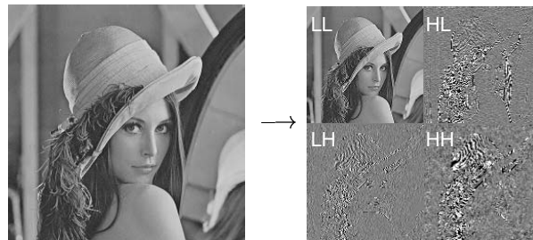
Figure 3 Wavelet transformation of the Lena image into LL, HL, LH, HH layers. The LL layer is a downsampled version of the original image and the HL, LH, and HH layers contain the information required to restore horizontal, vertical, and diagonal resolution, respectively.
