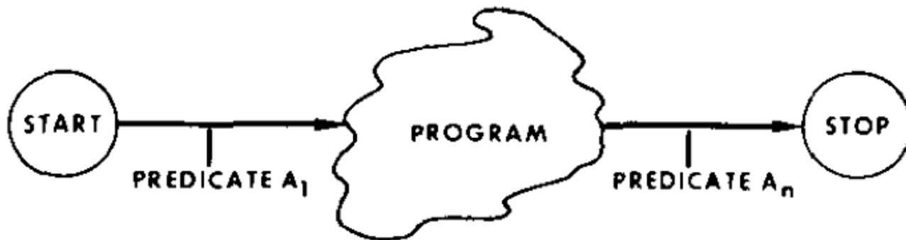
FIGURE 8. Predicates A_1 and A_n specify input-output behavior of a program.
