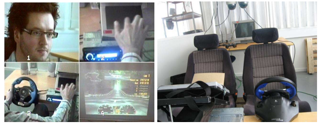
Figure 6. Frame from the laboratory video feed showing a participant driving the simulator while using gesture interaction (left). Setup in the driving simulator with force-feedback steering wheel and car seats (right).
