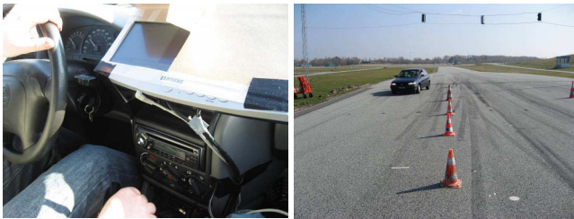
Figure 5. Vehicle setup with the touch interaction and gesture interaction players running off a touch screen (left). The car stereo (tactile interaction) is placed just below. Subject driving the vehicle used in the experiment (right).
