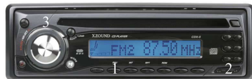
Figure 1. The conventional car stereo (Xzound CDX5) used for the tactile interaction. Play/pause is located at the lower middle part (1), skip forward/back is located in the lower right (2), and the volume is controlled via the knob to the left (3).
