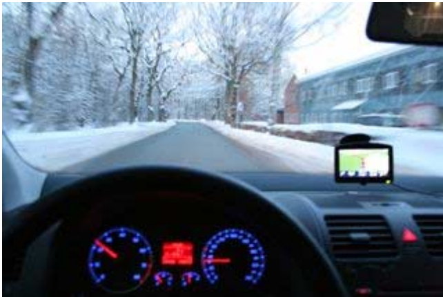
Figure 2. Experimental setup with the placement of the GPS system in the lower-middle area of the windscreen (as seen from the driver's point of view).
