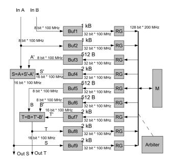
Fig. 1. Radar memory interface board
