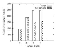
The throughput is roughly 75% of the throughput in Linux and this is because a overhead in virtual interrupts.
