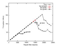
The throughput is less than 80% of the throughput in Linux.
