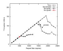
The throughput is only around 34% of the throughput in Linux.
