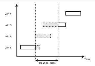
Figure: BT Device bouncing between AP 1, AP 2, and AP 3.
