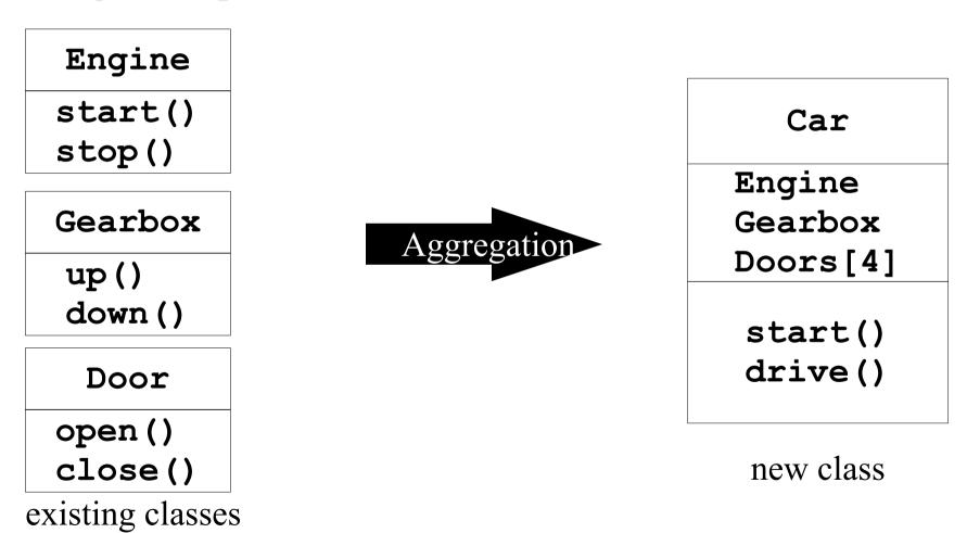
• Car "has-a" Gearbox and Car "has-an" Engine
